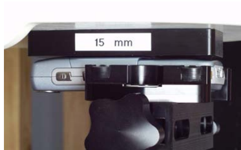
Photo of the device positioned for Body SAR measurement. The spacer was removed for the tests.
