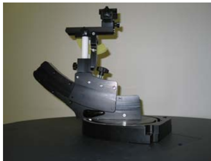
Device holder supplied by SPEAG
