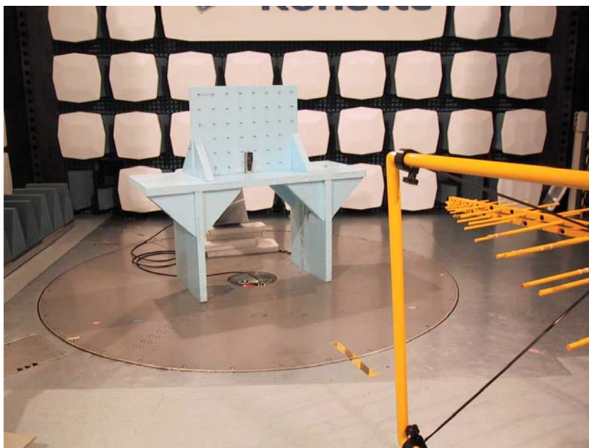
Picture 2: Radiated spurious emission measurement set-up for below 3 GHz measurements, EUT in vertical orientation
