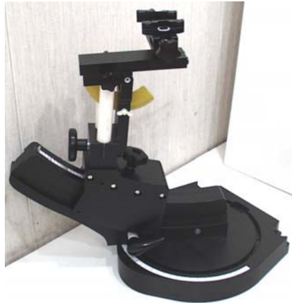
Device holder supplied by SPEAG
