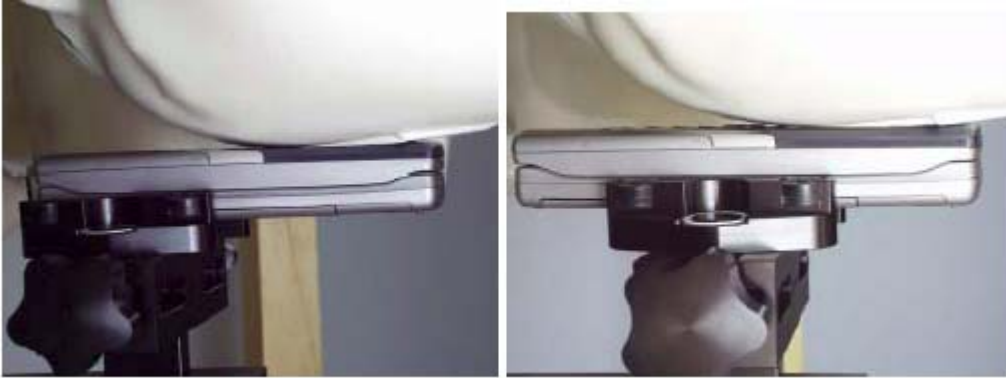
Photo of the device in “cheek” position, for GSM testing on the left and for WLAN on the right.
