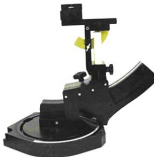
Device holder supplied by SPEAG
