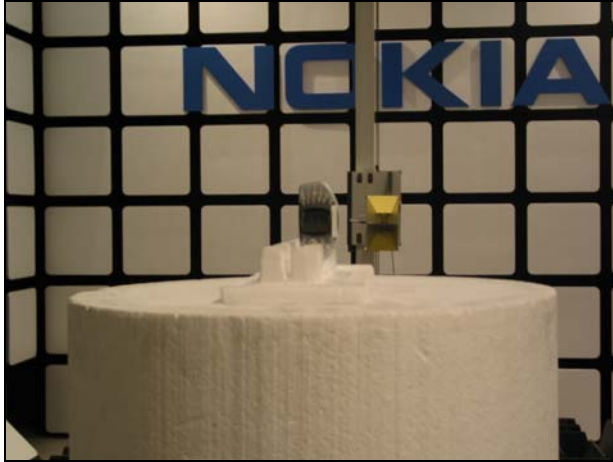
RF Output power measurement
