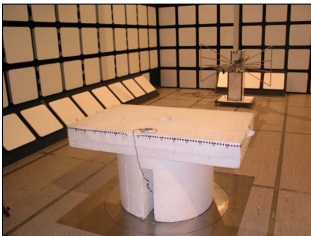
Radiated emission measurement
