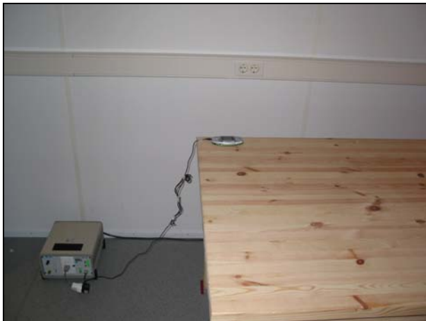
AC powerline emission measurement
