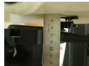
Figure 12. Body SAR Test Setup
