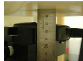
Figure 11. Mouth Face SAR Test Setup
