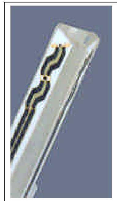
Inside view of ET3DV6 E-field Probe
