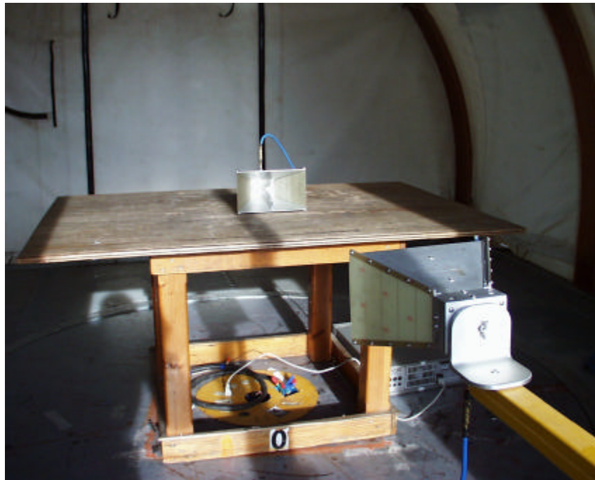
Above 1 GHz Substitution Method Setup
