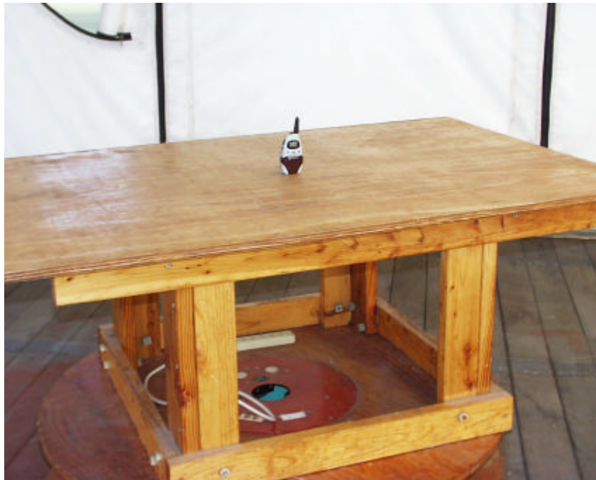
Radiated Emission Setup 30 – 1000 MHz
