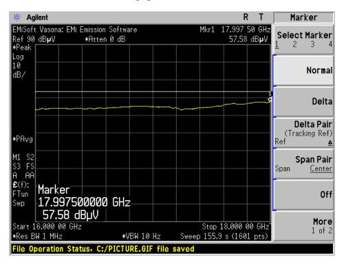
Note: above plot shows reduced VBW to make average measurements comparing to average limits and thus show compliance in range of 16-18GHz
