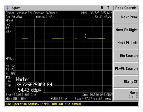
Note: above plot shows reduced VBW to make average measurements comparing to average limits and thus show compliance in range of 39-40 GHz
