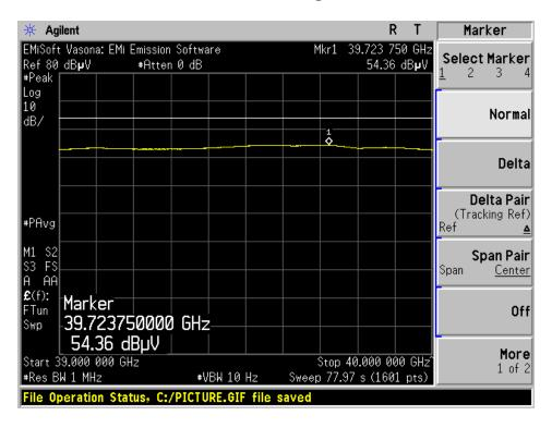
Note: above plot shows reduced VBW to make average measurements comparing to average limits and thus show compliance in range of 39-40 GH
