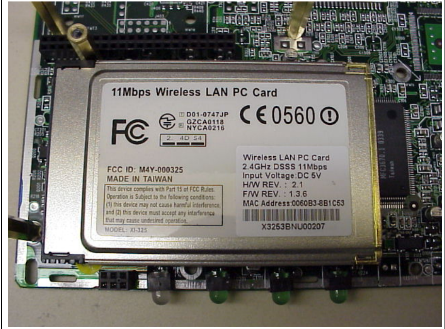
WLAN Module Close up View
