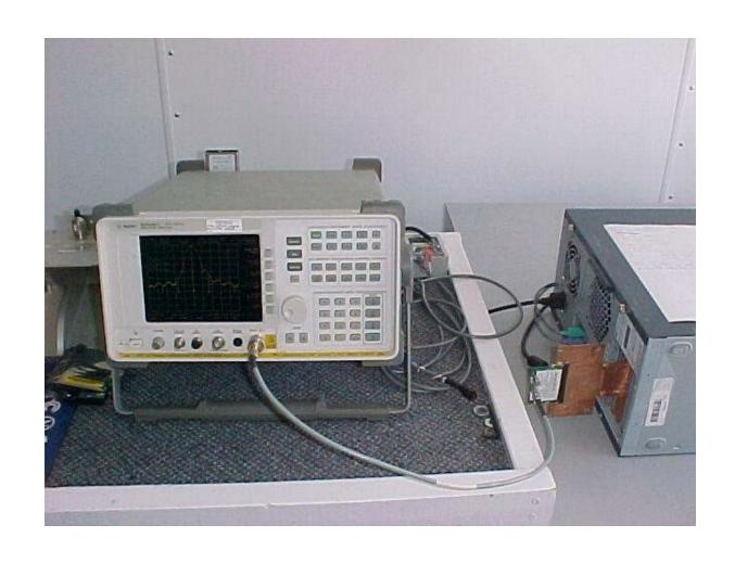
Conducted Emissions at Antenna Terminal Setup
