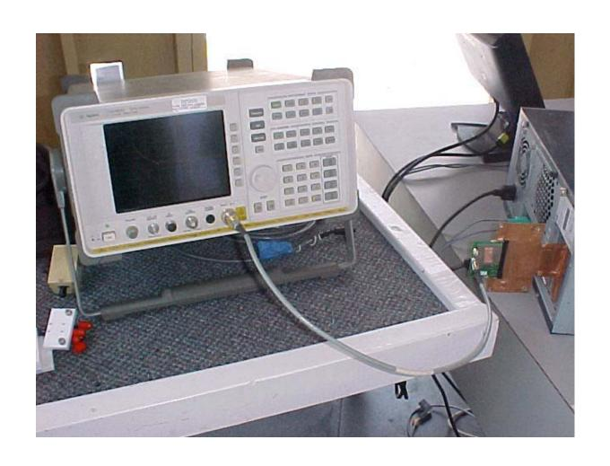
Conducted Emissions at Antenna Terminal Setup
