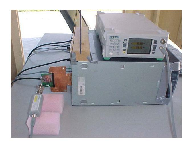
Maximum Peak Output Power Measurement Setup
