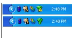
Authentication failed. Not able to authenticate with wireless network. Green icon with a yellow warning triangle
