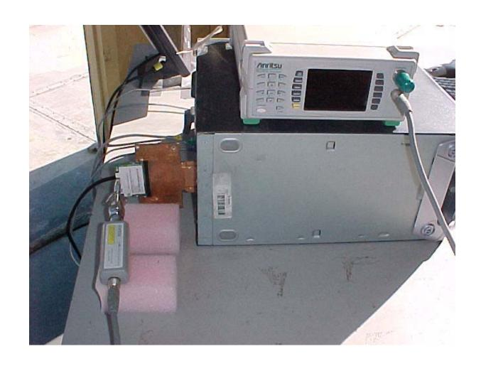
Maximum Peak Output Power Measurement Setup
