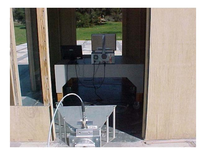
Radiated Emissions Measurement (1-26.5 GHz) (Rear View) Setup
