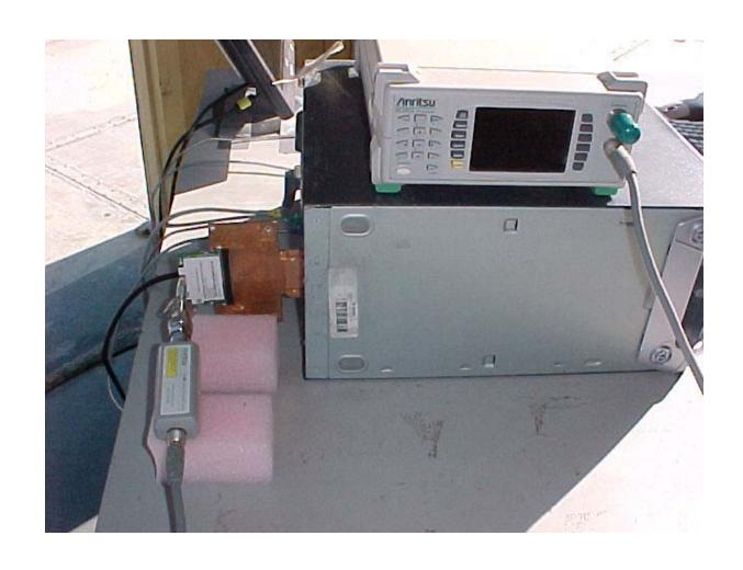
Maximum Peak Output Power Measurement Setup
