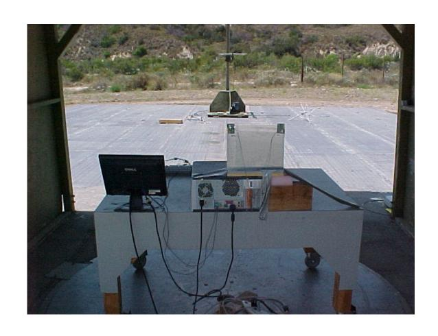
Radiated Emissions Measurement (30-100 MHz) (Rear View) Setup
