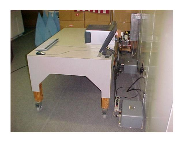
AC Conducted Emissions Measurement (Rear View) Setup
