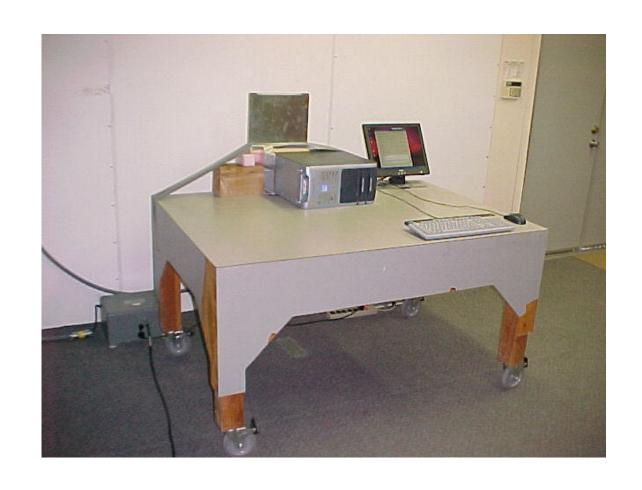
AC Conducted Emissions Measurement (Front View) Setup
