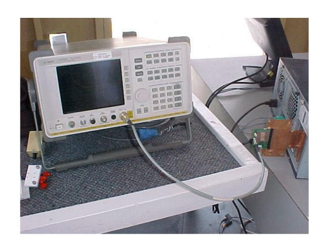
Conducted Emissions at Antenna Terminal Setup
