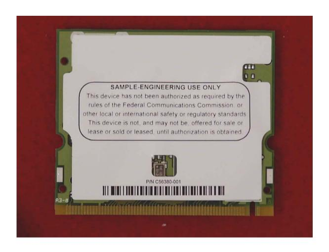
Bottom View of the WLAN Transmitter "With Insulation"
