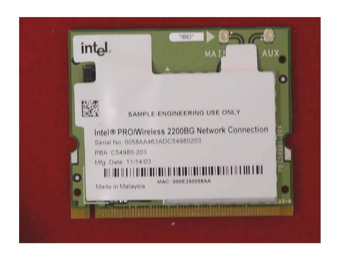
Top View of the WLAN Transmitter "With Insulation"
