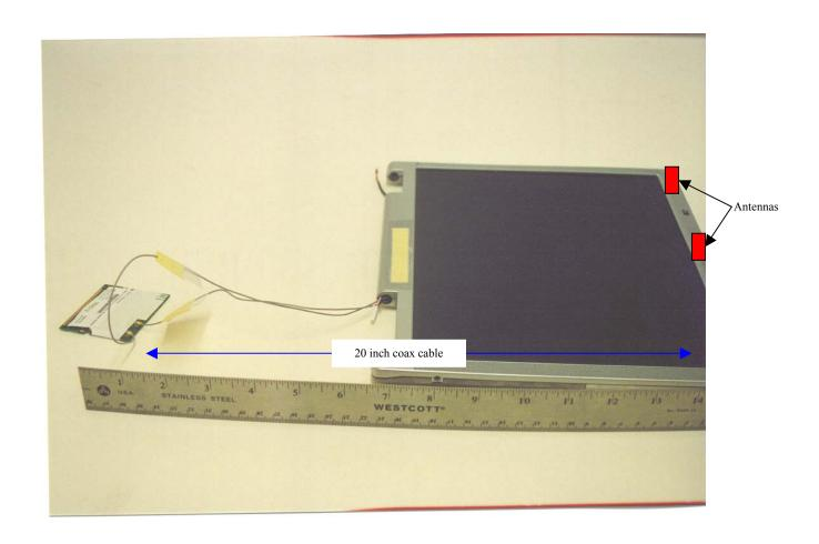
View as Tested Inside Laptop LCD "CF-73 Antennas"
