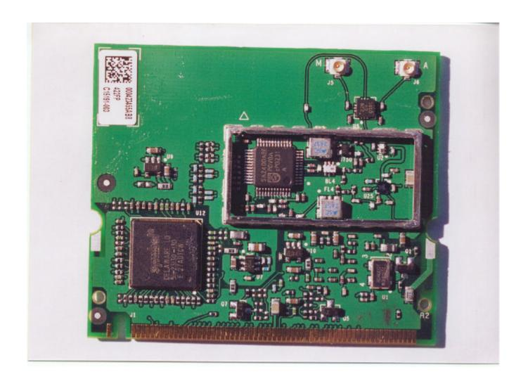
Top View "Shielding removed"
