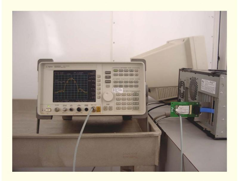
Conducted Emissions at Antenna Terminal Setup
