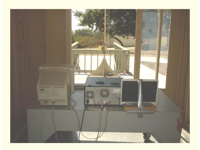
Radiated Emissions Measurement (Rear View) Setup
