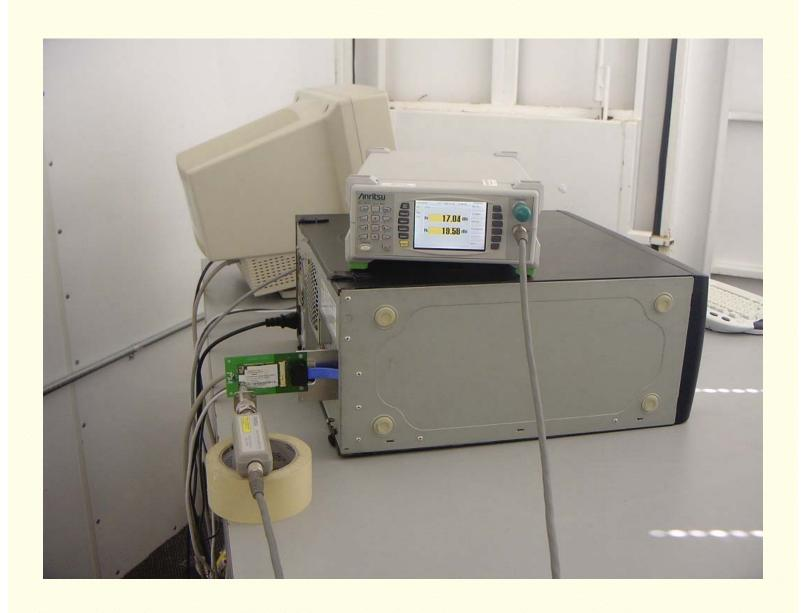
Maximum Peak Output Power Measurement Setup
