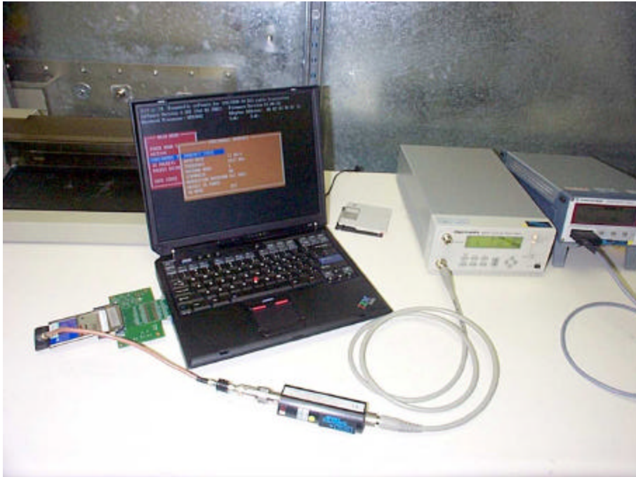
Intel – 2011B LAN CF Card Maximum Peak Output RF Power Measurement (Conducted)
