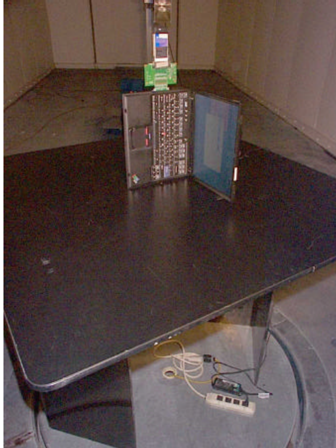
Testing for Radiated Emissions from Transmitter in Restricted Bands Close View
