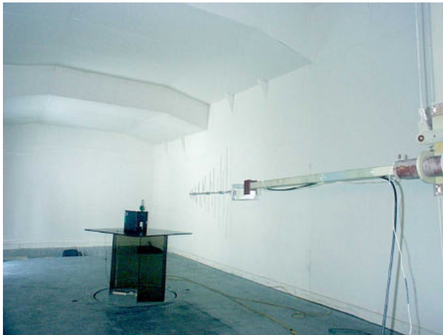
Testing for Radiated Emissions from Transmitter in Restricted Bands Frequency Range: 200 MHz – 1 GHz
