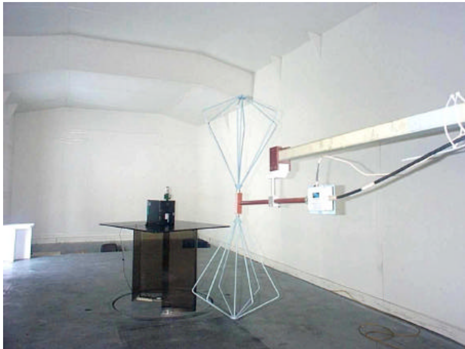
Testing for Radiated Emissions from Transmitter in Restricted Bands Frequency Range: 30 MHz – 200 MHz
