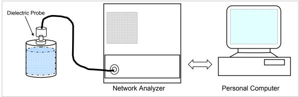
Set-up for liquid parameters check
