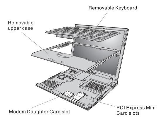
**Attention:** The ThinkPad X60 Series computer contains an authentication mechanism You can install or remove each wireless feature by yourself. If you install an unauthorized wireless adapter that is not approved for use in the ThinkPad X60 Series computer, the computer will not start, but only displays an error message and emits beeps.
