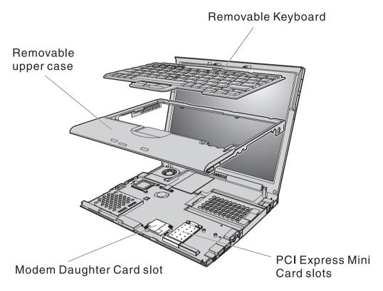
**Attention:** The ThinkPad X60 Series computer contains an authentication mechanism If you install an unauthorized wireless LAN Mini PCI Express Card that is not approved for use in the ThinkPad X60 Series computer, the computer will not start, but only displays an error message and emits beeps.
