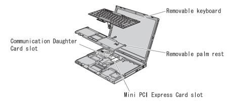
**Attention:** The ThinkPad T60 Series computer contains an authentication mechanism You can install or remove each wireless feature by yourself. If you install an unauthorized wireless adapter that is not approved for use in the ThinkPad T60 Series computer, the computer will not start, but only displays an error message and emits beeps.
