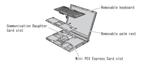
**Attention:** The ThinkPad T60 Series computer contains an authentication mechanism If you install an unauthorized wireless LAN Mini PCI Express Card that is not approved for use in the ThinkPad T60 Series computer, the computer will not start, but only displays an error message and emits beeps.
