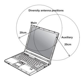
**Note:** The transmission diversity function is implemented for the models AR5BXB6 and WM3945ABG. The function does not emit radio frequencies simultaneously from both antennas. One of the antennas is selected automatically or manually (by users) to have good quality of radiocommunication.
