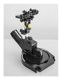
The DASY device holder is designed to cope with the different positions given in the standard. It has two scales for device rotation (with respect to the Head axis) and device inclination (with respect to the line between the ear reference points). The rotation center for both scales is the ear reference point (ERP). Thus the device needs no repositioning when changing the angles.
