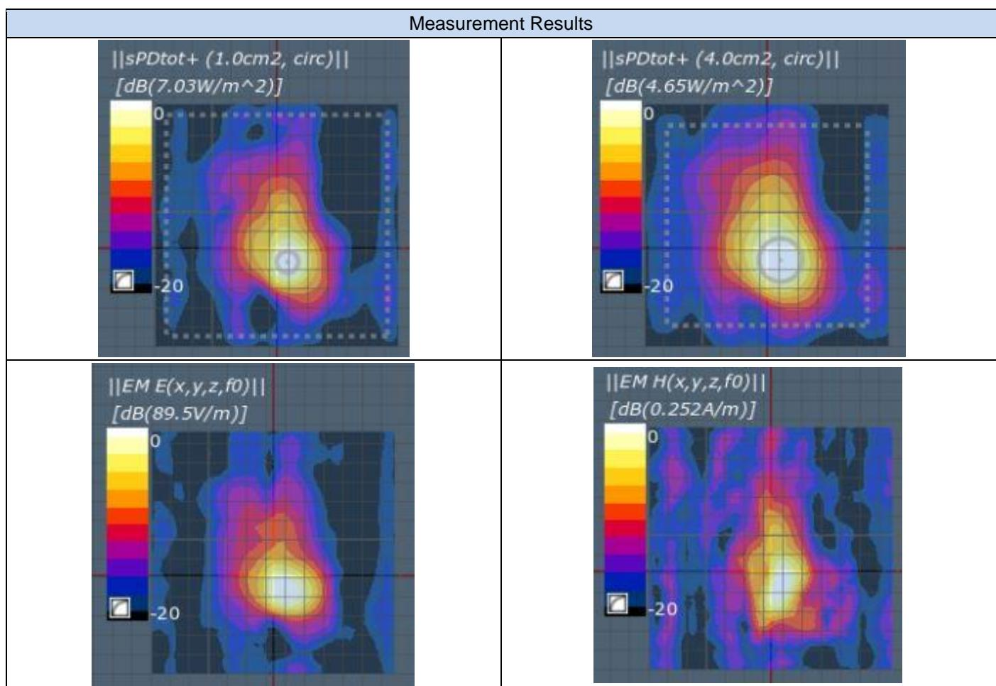
**16.U-NII-6 - 802.11ax/be160, CH111, Main WNC – Position Laptop (PD)****DUT: P184G BE201D2W; Type: PIFA****Signal Source: modulation Custom Channel for 802.11ax/be, level 14.50dBm.**Medium parameters used:  $\sigma = 0 \text{ S/m}$ ,  $\epsilon_r = 1$ ;  $\rho = 0 \text{ kg/m}^3$
