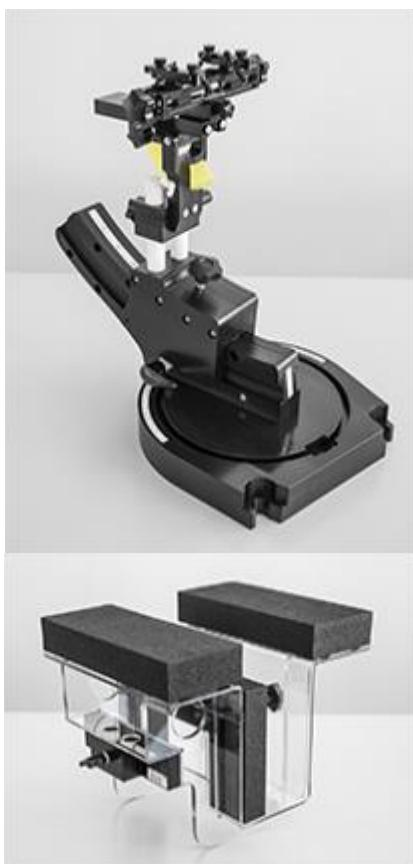
The DASY device holder is designed to cope with the different positions given in the standard. It has two scales for device rotation (with respect to the body axis) and device inclination (with respect to the line between the ear reference points). The rotation center for both scales is the ear reference point (ERP). Thus the device needs no repositioning when changing the angles.
