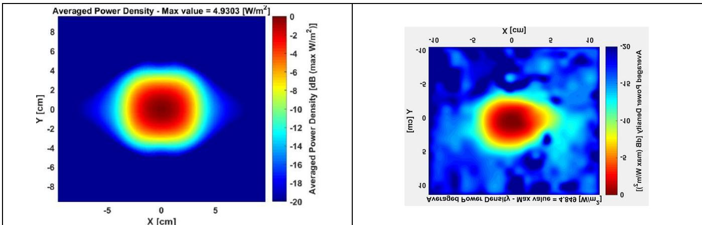
The plots below show the comparison between the numerical modeling and the system check results in terms of normalized E-field distribution and the 1D variation along the two axis of the maximum.
