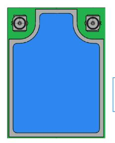
The device is considered to be too small for the label since it is impracticable to label with a font side that is four-points or larger. The FCC ID and IC ID is instead placed in the users manual as allowed by KDB 784748. External host labeling is still required once integrated into host.
