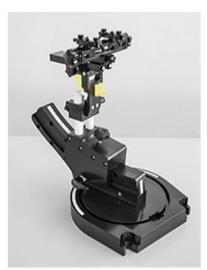
The DASY device holder is designed to cope with the different positions given in the standard. It has two scales for device rotation (with respect to the body axis) and device inclination (with respect to the line between the ear reference points). The rotation center for both scales is the ear reference point (ERP). Thus the device needs no repositioning when changing the angles.
