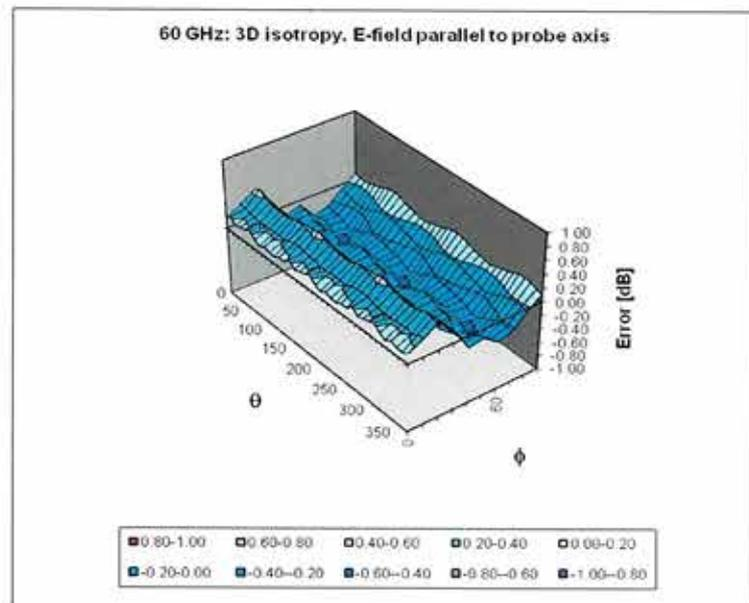
Probe isotropy for  $E_{tot}$ : probe rotated  $\phi = 0^\circ$  to  $360^\circ$ , tilted from field propagation direction  $\vec{k}$
