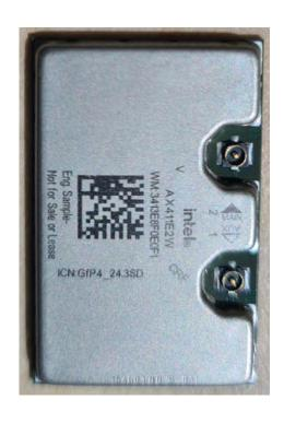
Note: Due to the small device size 16mm x 25mm it is too small to imprint the FCCID and IC ID on the module. The font size required would need to be < size 4 font and is considered to require magnification for legibility. The ID's will be placed in the Information Guide. External host labeling is still required once integrated into host.
