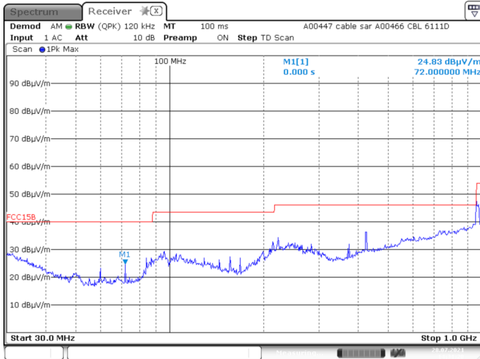
Plot 1: Pre-scan plot with peak detector. Radiated emissions from 30 MHz to 1000 MHz 5GHz + BT mode
