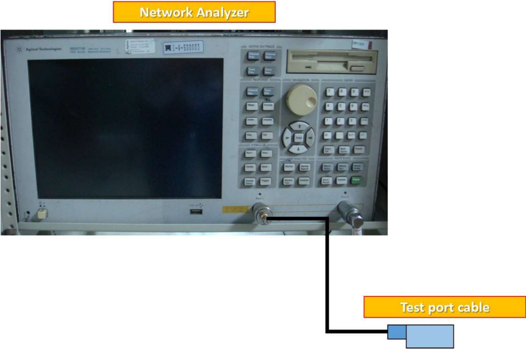
Figure 1. The schematic diagram for measuring VSWR
