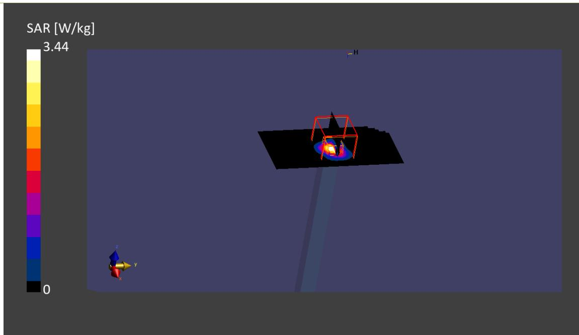
**14. U-NII-5 - 802.11ax160, CH15, Main – Position Back Face (PD)****DUT: Lenovo 500e Chromebook Gen 4s w AX211NGW; Type: PIFA****Signal Source: modulation Custom Channel for 802.11ax, level 11.50dBm.**Medium parameters used:  $\sigma = 0 \text{ S/m}$ ,  $\epsilon_r = 1$ ;  $\rho = 0 \text{ kg/m}^3$
