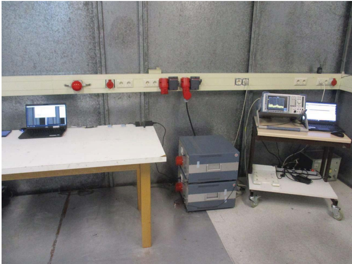
Photo 5: Photograph conducted emissions 0.15-30 MHz
