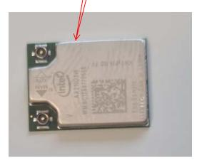
FCC ID: PD9AX210D2 IC: 1000M-AX210D2 The device is considered to be too small for the label since it is impracticable to label with a font side that is four-points or larger. The FCC ID is instead placed in the users manual as allowed by KDB 784748 and as allow by ISED previously on this form factor.
