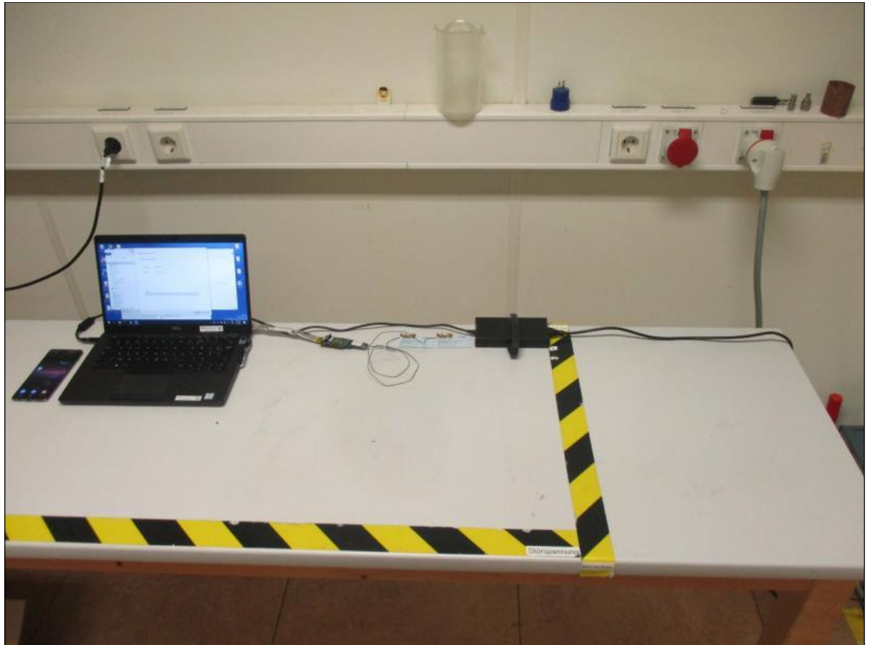
42 Picture 1: Conducted voltage emissions
