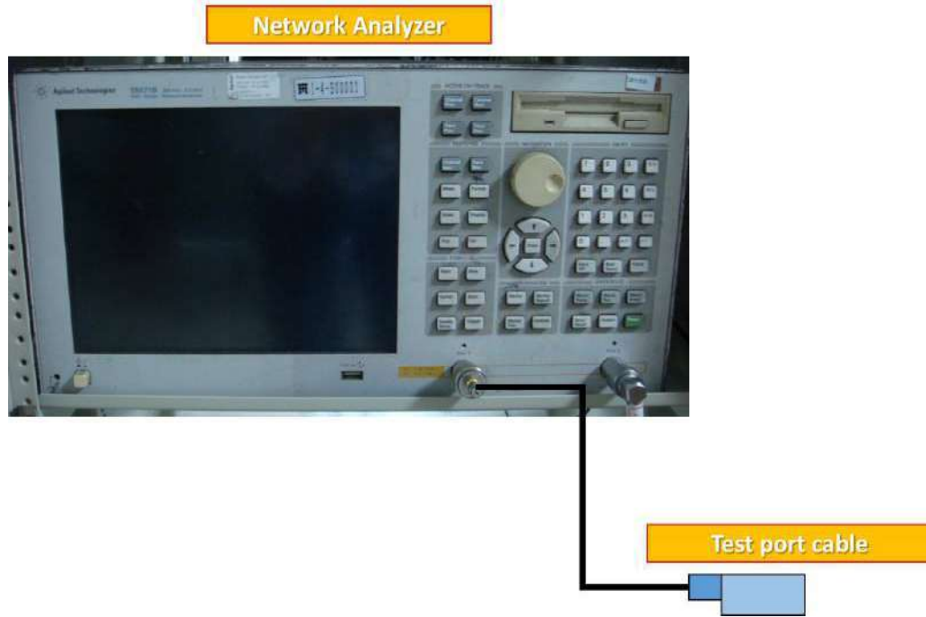
Figure 1. The schematic diagram for measuring VSWR
