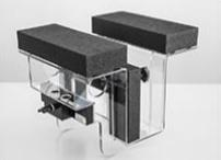
The DASY device holder is designed to cope with the different positions given in the standard. It has two scales for device rotation (with respect to the body axis) and device inclination (with respect to the line between the ear reference points). The rotation center for both scales is the ear reference point (ERP). Thus the device needs no repositioning when changing the angles.
