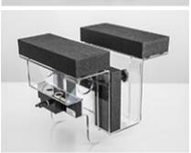
The DASY device holder is designed to cope with the different positions given in the standard. It has two scales for device rotation (with respect to the body axis) and device inclination (with respect to the line between the ear reference points). The rotation center for both scales is the ear reference point (ERP). Thus the device needs no repositioning when changing the angles.
