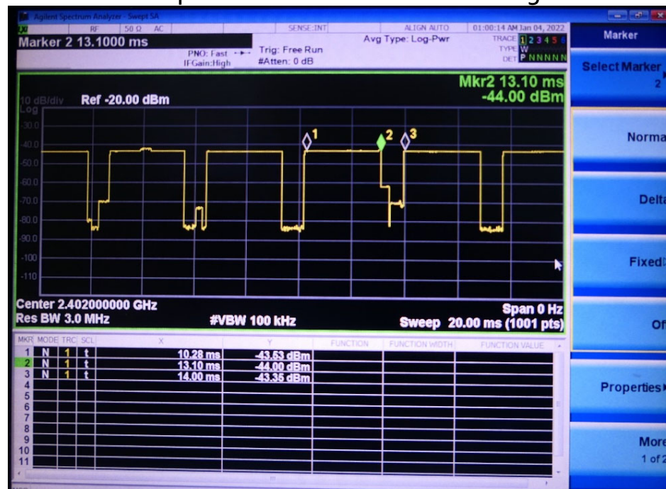
Time-domain plot for Bluetooth transmission signal
