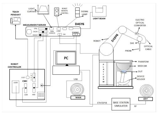
The DASY system for performing compliance tests consists of the following items:
