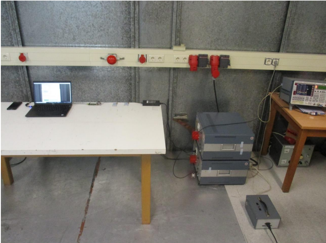
Photo 4 Photograph conducted emissions 0.15-30 MHz
