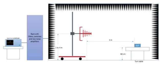
Radiated Setup 1 GHz - 18 GHz
