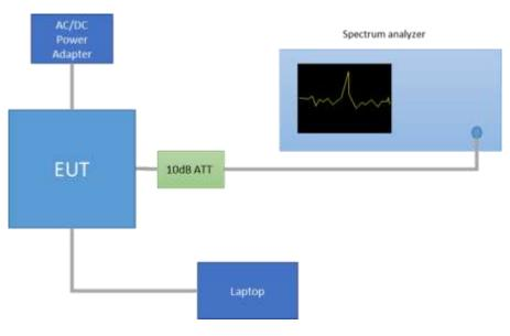
Radiated Setup 30 MHz- 1 GHz
