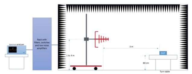
Radiated Setup 1 GHz - 18 GHz
