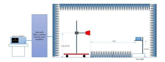
Radiated Setup 18 GHz - 26.5 GHz
