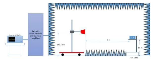
Radiated Setup 18 GHz - 26.5 GHz
