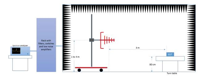
Radiated Setup 1 GHz - 6.4 GHz
