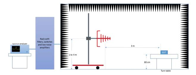
Radiated Setup 1 GHz - 6.4 GHz
