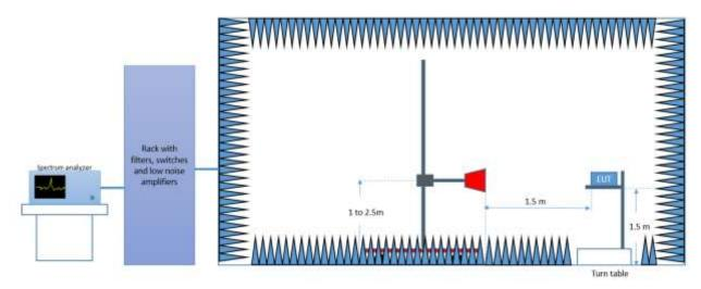
Radiated Setup 6.4GHz - 18 GHz
