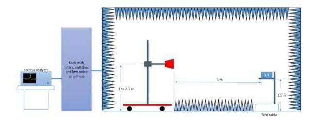
Radiated Setup 6.4GHz - 18 GHz
