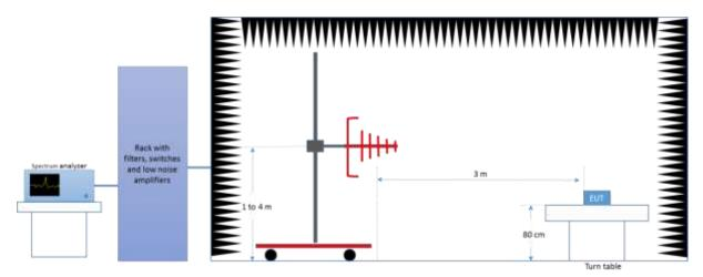
Radiated Setup 1 GHz - 6.4 GHz
