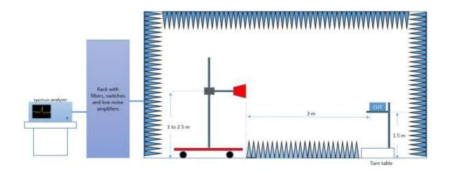
Radiated Setup 6.4GHz - 18 GHz
