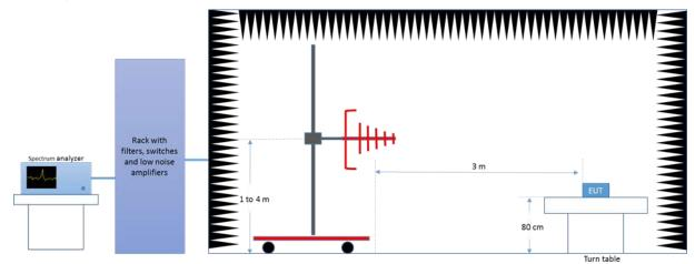
Radiated Setup 1 GHz – 6.4 GHz
